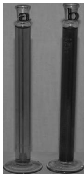
Figure 2 Photograph of GNs and modified GN dispersions in distilled water after standing for 1 h: (a) GN-g-PSt and (b) pristine GNs.
